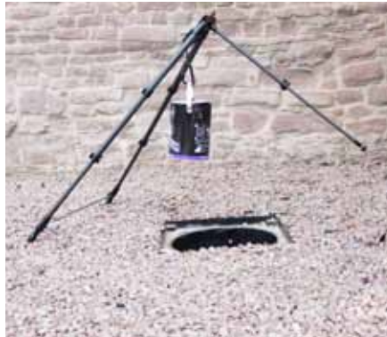
The A-Frame has a third, shorter, detachable leg for added stability on uneven ground or where a tether point is not available.
