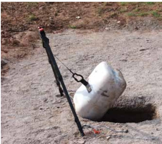
The legs can also be tethered using metal or plastic anchor pegs depending on the ground conditions.
