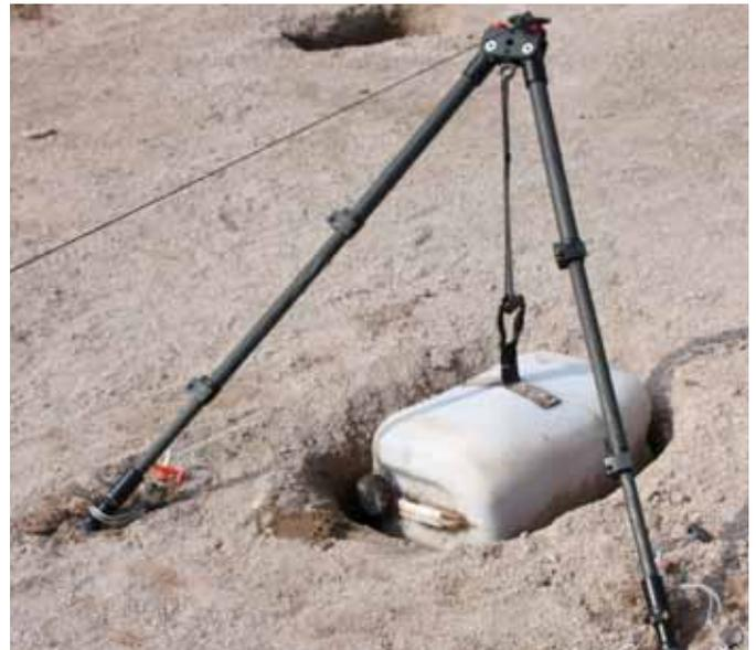
The legs can be locked in three positions: vertical, semi-spread, and fully spread.
