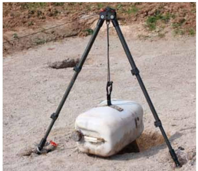
The operator can choose to deploy the A-Frame with steel points on the feet or rubber grips to assist with stability.
