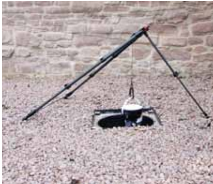
The A-Frame has a third, shorter, detachable leg for added stability on uneven ground or where a tether point is not available.
