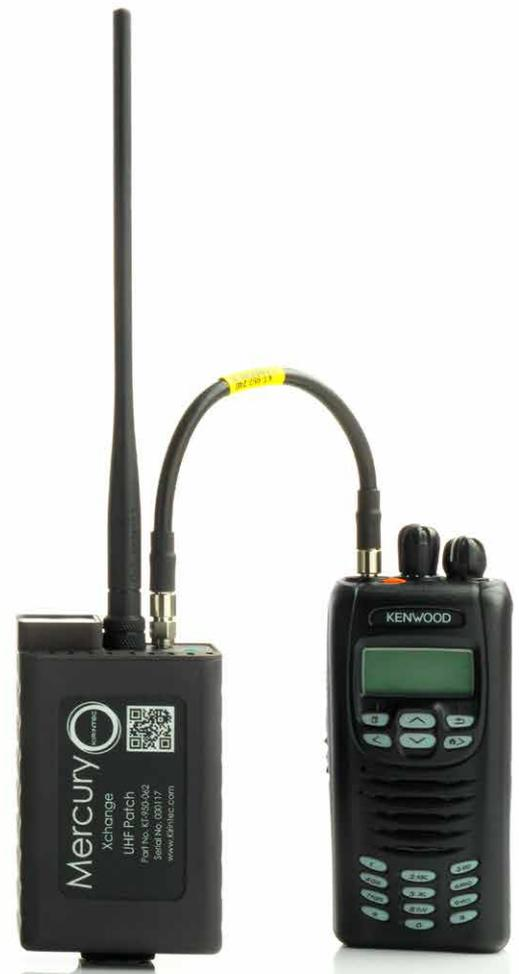
*Xchange: allows unbroken communications while jamming*
