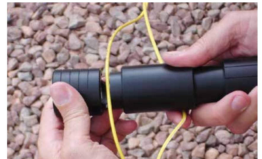
Cuts multi-stranded copper core wire up to 7mm diameter
